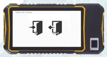
7.0 inch TFT-LCD (1024x600) touch screen with backlight Cortex A7 1.3GHz quad Android OS 4.4.3 industrial tablet Wi-Fi/3G, Camera, Bluetooth, GPS ready 1GB RAM, 16GB ROM, MicroSD (max 32GB expansion) IP65 Weatherproof 1.5/4.6ft drop tested Rechargeable li-ion polymer, 3.7V, 10000mAh 208mm (H) x 130mm (W) x 20 mm (D) ±2mm Exclude wall mount bracket
